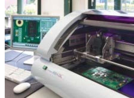
The Marantz 22X DL assists in the automated optical inspection of printed circuit boards.
